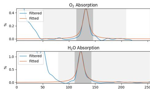
Oxygen and water vapor absorption signals obtained from the infant No.25 with measurement performed on the left side of the chest with DP in the armpit and LS in a 3<sup>rd</sup> position (LS3)
